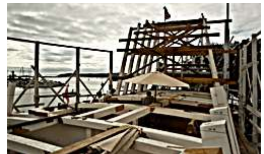
The rising sterncastle, deck beams and stringers of the San Salvador's main deck.
